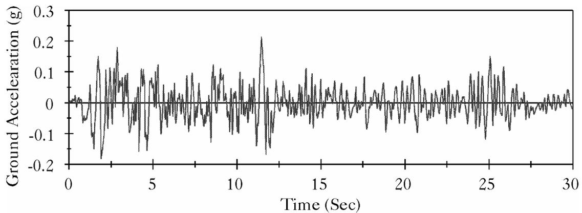
**FIG. 3. East West Component of the 1940 El-Centro Earthquake**
