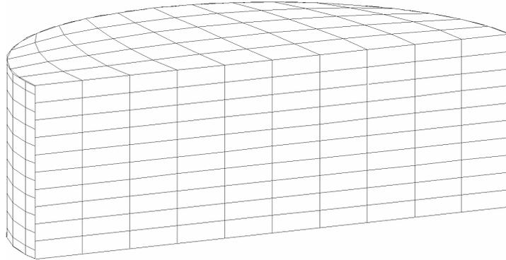
**FIG. 1. Finite Element Mesh for the Coupled Liquid-Broad Tank System**
