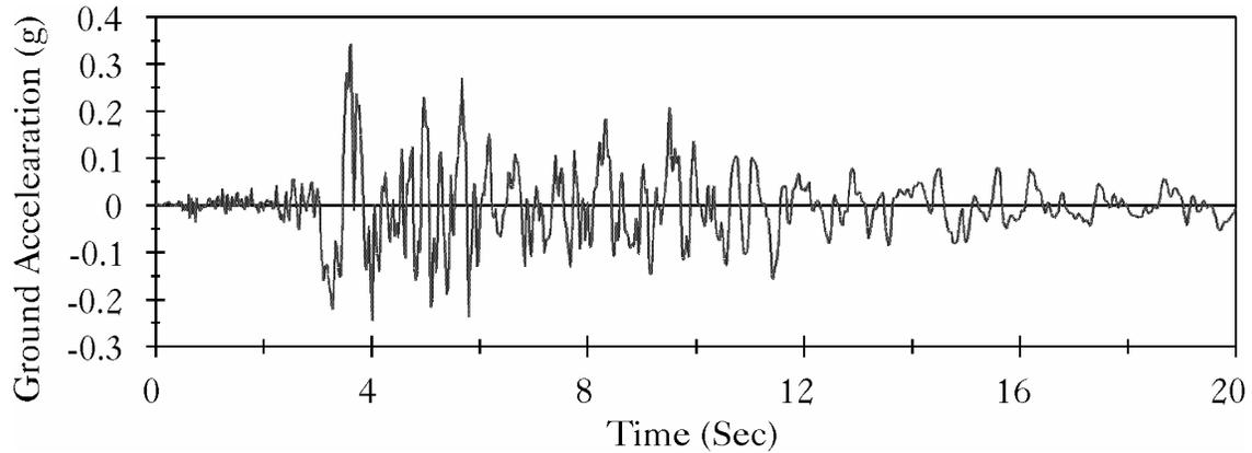
**FIG. 4. Northridge Earthquake Measured at Arleta Site**
