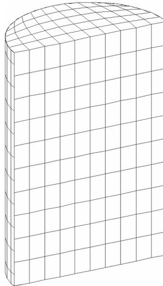
**FIG. 2. Finite Element Mesh for the Coupled Liquid-Tall Tank System**
