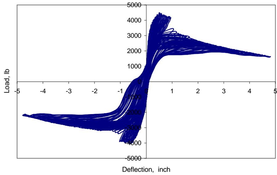
Figure 8: Load-Deflection Curve of the Retrofitted Wall
