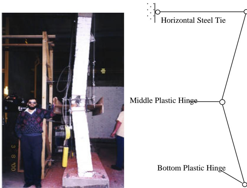
Figure 7: Failure Mechanism of the Repaired Wall
