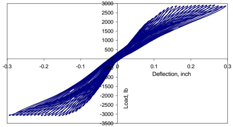
Figure 4: Load-Deflection Curve of the Un-Injected Wall
